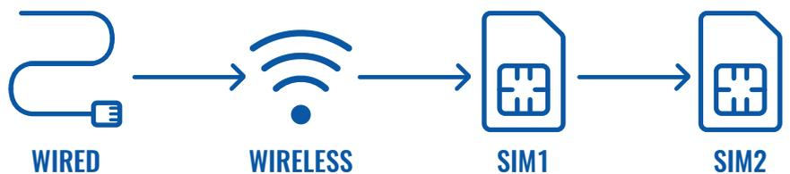
ATMs are a good example where having a single connectivity option is out of the question due to the risks of downtime. Nowadays, the complete majority of ATMs across the globe are using industrial cellular routers to ensure connection continuity between ATMs and central systems of the bank, and leveraging multiple connectivity sources at the same time, including wired and cellular.
